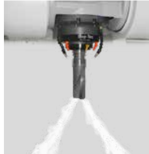
Internal tool cooling
