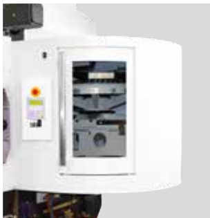
Tool magazine HSK-A/T100: 30 tools HSK-A/T63: 45 tools
