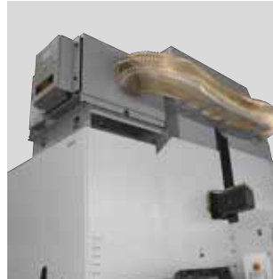
Suction removal of mist
